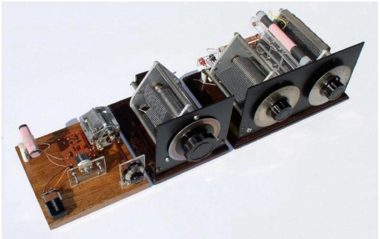
In this photo, the 1-MPF 102 JFET BFO is on the left. At center is a 1000 pF variable capacitor shunted across the BFO's tuning capacitor to get to low frequencies (the BFO was originally designed to cover the mediumwave band). The two-dial unit to the right is a double-tuned LF crystal set. It is a series-tuned front-end design loosely coupled to a parallel-tuned secondary detector section.
