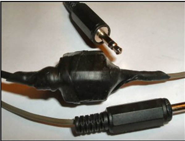
Above: the final assembly, wrapped in self- amalgamating tape for extra strength and insulation!
